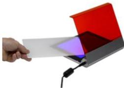
The proBLUEVIEW transilluminator is ideal for safely imaging DNA gels stained with fluorescent stains such as RunSAFE, SYBR Safe, Gold and Green, GelGreen and UltraSafe blue as well as protein gels stained with Coomassie, Silver stains.
