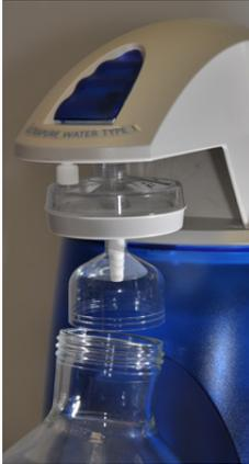
Measure the total volume of water (in Liters) dispensed from the system using a 1 L graduated cylinder.
