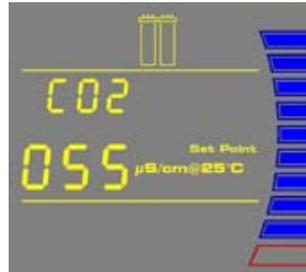
If Conductivity Units are chosen in C01, then the Setpoint can be adjusted from 0.999 μS/cm @25 °C to 0.055 μS/cm @25 °C.
