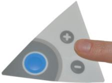
Press the "+" or "-" Button to adjust the exact amount of Product Water (in Liters) needed. Pre-set volumes of water can be adjusted from 0.25 L to 9.75 L in 0.25 increments.
