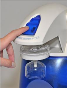
Press the Dispensing Button once. The system will dispense water. The Display will show the amount of water dispensed and the Product resistivity.
