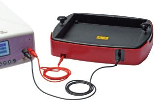
corrosion and so provide many years of trouble free use. Uniform heat dispersion across the blot sandwich ensures stable transfer times and no heat induced sample loss or transfer distortions.
