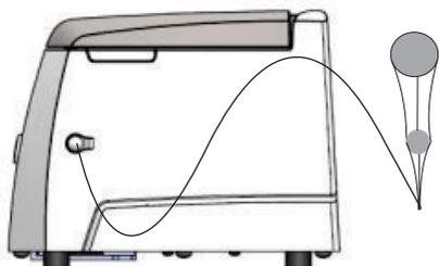
Disconnect the centrifuge from the main supply. Wait until the rotor comes to a stillstand (this may take some time). Once the rotor has stopped, pull out the emergency lid release as shown in the figure.
