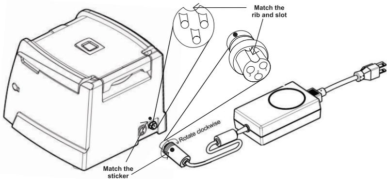
4. If matched correctly the plug will go in easily without much force (do not try to force the plug in if it is not matched properly). Once the plug is inserted into position, turn the loose upper ring clockwise to tighten & to secure the fitment.
