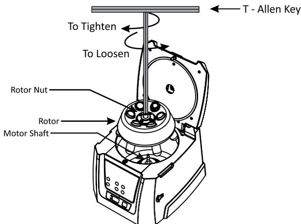
The rotor of the centrifuge is pre-installed. In case of any spillage, remove the rotor as shown in the figure above to clean the rotor and its chamber thoroughly.
