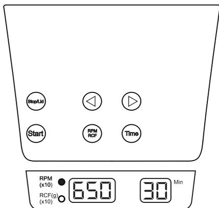
1. To set the speed press the RPM/RCF button first, then with the use of increment & decrement buttons to set the desired speed.
