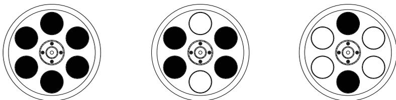
2. The samples in the tubes should be of equal volume. To achieve a balanced condition of the 6 "Tube Holders are mandatory to place inside the rotor whether 2, 3, 4 or 6 / 8 tubes are being used
